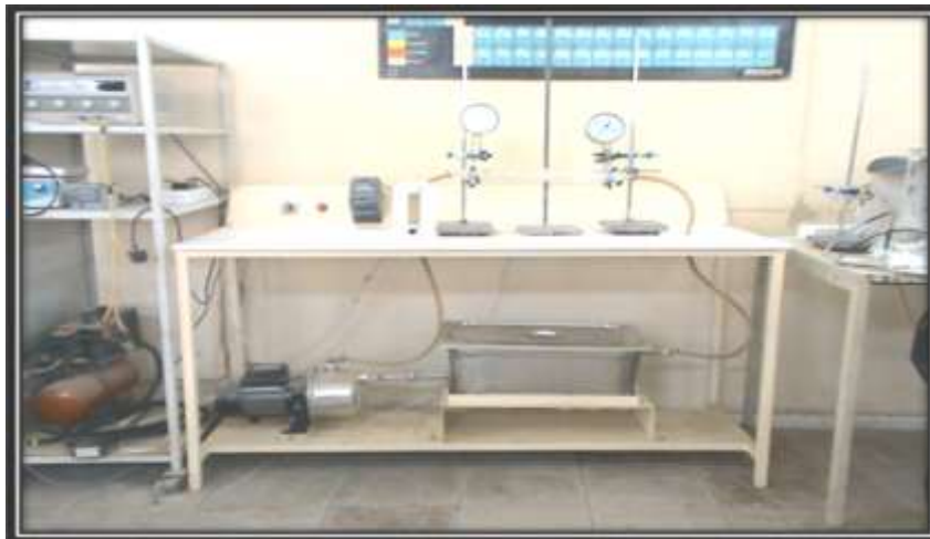
Fig .2.The experimental system of the convective heat transfer and flow characteristics for nanofluids
